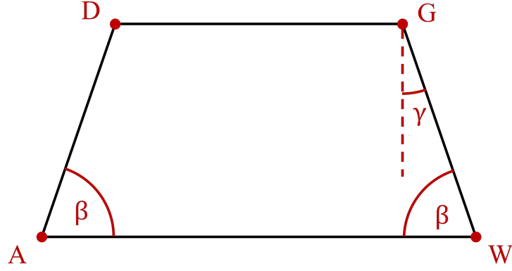
Figure 3.25: The regular trapezoid ADGW which validates Cartmell et al.'s substitution of \gamma = \frac{\pi}{2} - \beta .
